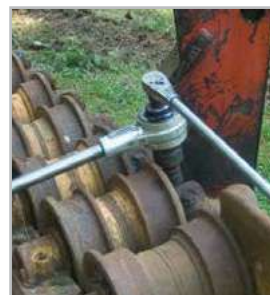
Torque multiplier used on tracks
