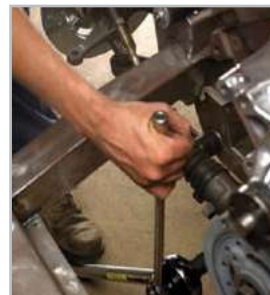
Torque multiplier used in inaccessible areas
