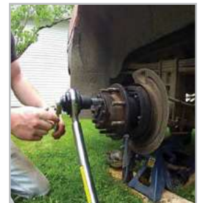
Torque multiplier used for lug nuts
