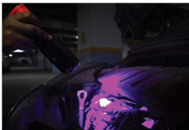
UV light for detecting engine oil leakage, gas leakage, crack in welding jobs in industrial, automotive, HVAC applications
