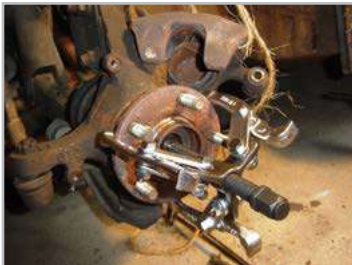
3 Jaw Puller used for removing tyre hub
